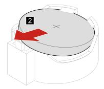
Note: After installing a new coin-cell battery, reset the system date and time in the UEFI BIOS menu.
